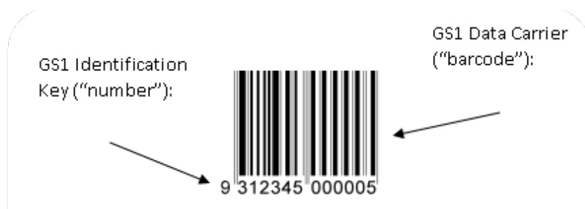
Figure 6: GTIN-13 vs. EAN-13
