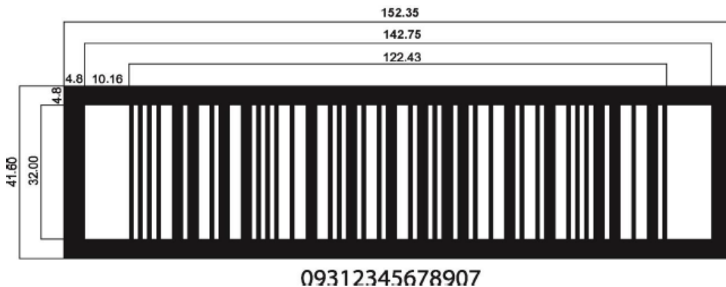
Figure 33: Example of a ITF-14 barcode at an X-Dimension of 1.02mm
