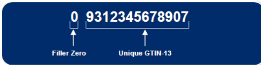
Figure 18: structure of GTIN-13 with a filler zero
