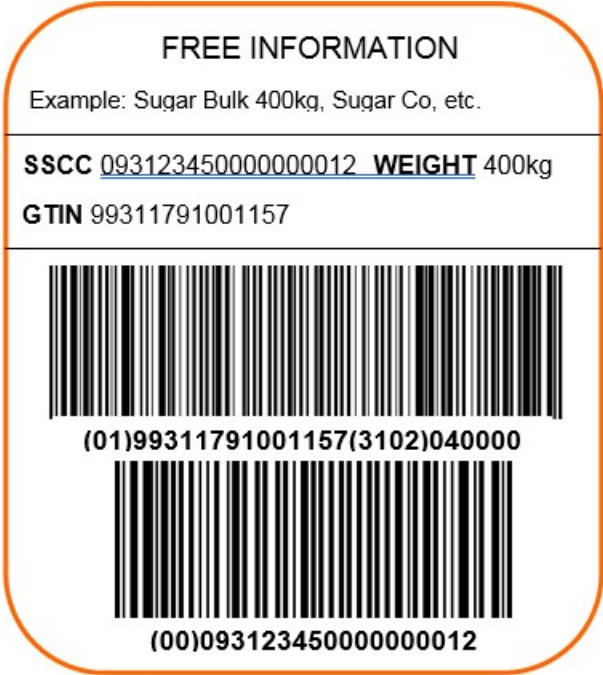
Figure 49: Example of a GS1 Logistics Label Format variable weight logistics unit containing the same product
