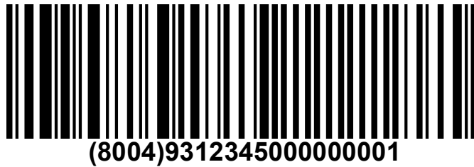
Figure 9: Global Individual Asset Identifier, AI (8004), represented in a GS1-128 Barcode
