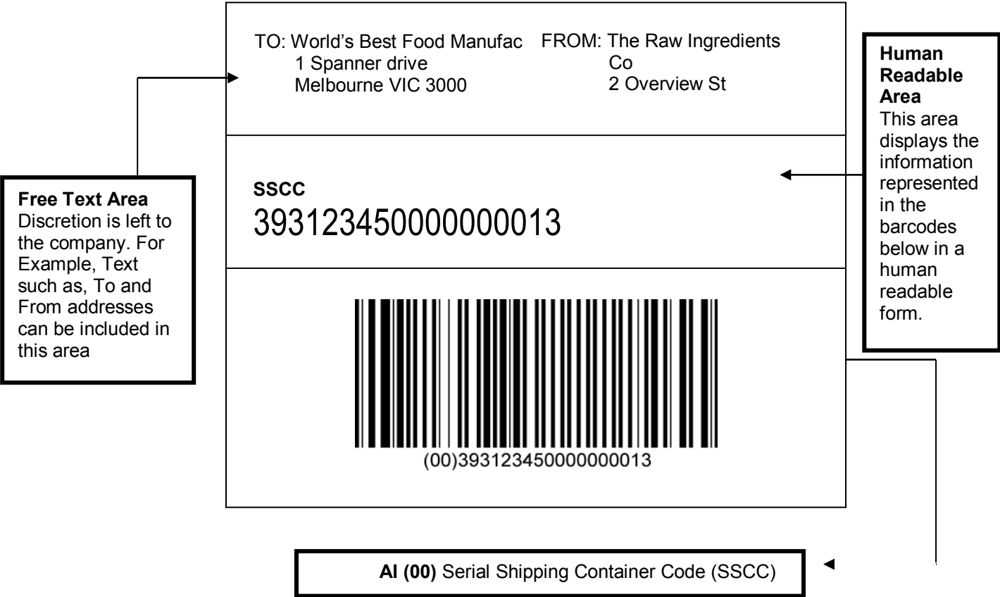
Figure 48: Example of a GS1 Logistics Label Format mixed trade items with different Customer Purchase Order Numbers and where full EDI is applicable
