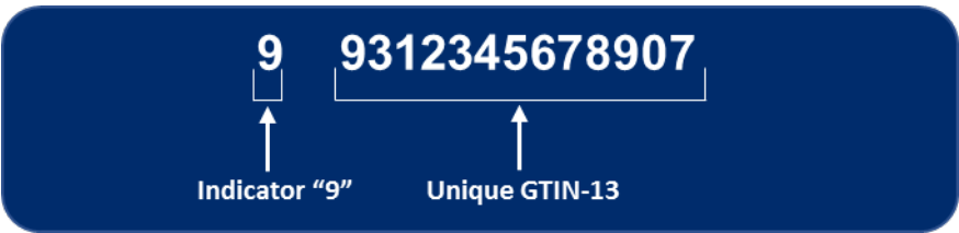
Figure 20: structure of a Variable Measure GTIN-14
