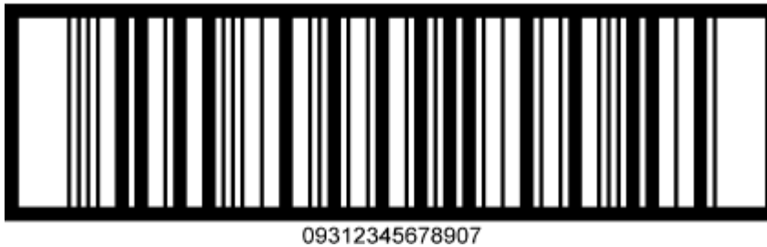
Figure 11: Example of an ITF-14 Barcode representing a GTIN-13 with a filler zero
