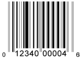
Figure 13: Example of a UPC-A Barcode representing the GTIN-12
