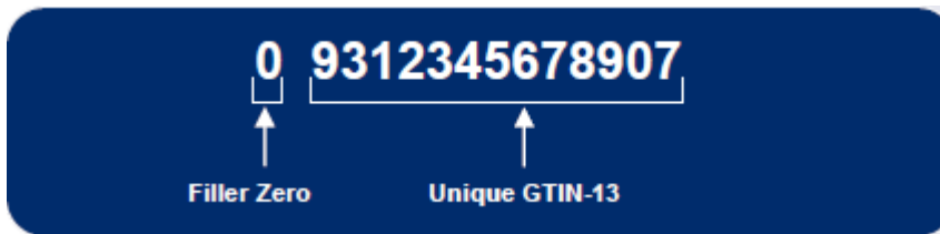
Figure 11: Example of an ITF-14 Barcode representing a GTIN-13 with a filler zero
