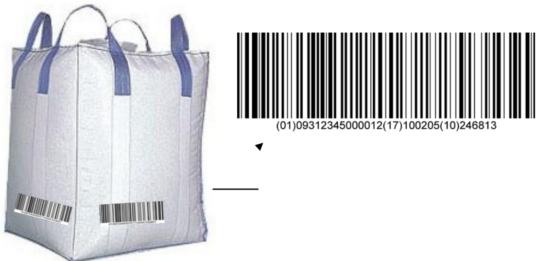
Figure 19: example of a GTIN-13 with a filler Zero for a bulk trade item. This is the base unit.
