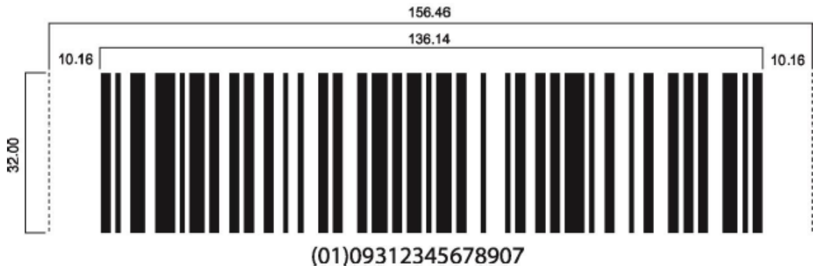
Figure 34: Example of a GS1-128 barcode at an X-Dimension of 1.02mm
