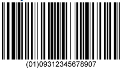
Figure 12: Example of a GS1-128 Barcode representing a GTIN-13 with a filler zero
