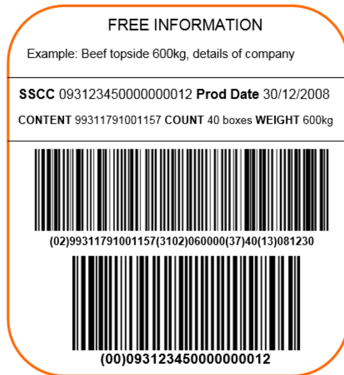
Figure 50: Examples of a GS1 Logistics Label Format Homogenous logistic unit containing variable weight product. All items on the logistic unit must be the same
