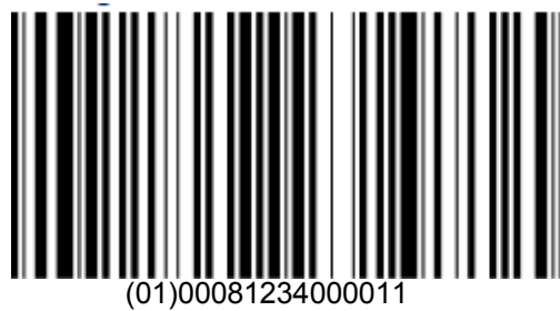
Figure 15: Example of a GS1-128 Barcode representing a GTIN-12 with two filler zeros
