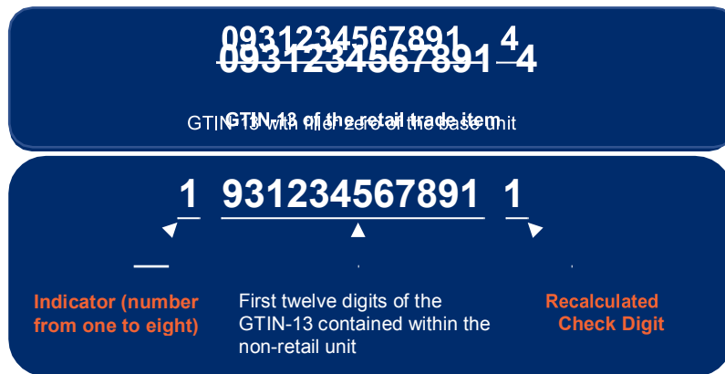
Figure 27: structure of GTIN-14 based on GTIN-13 with filler zero
