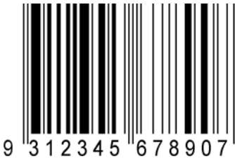
Figure 10: Example of an EAN-13 Barcode representing the GTIN-13
