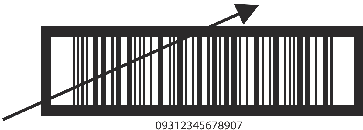
Figure 29 Example of a Skewed Scanning Beam
