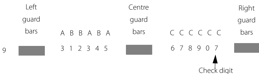
Figure 10 - EAN-13 Permutation for Bar Code Digit Positions
