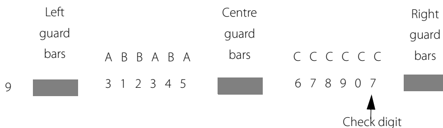
Figure 4 - EAN-13 Permutation for Bar Code Digit Positions
