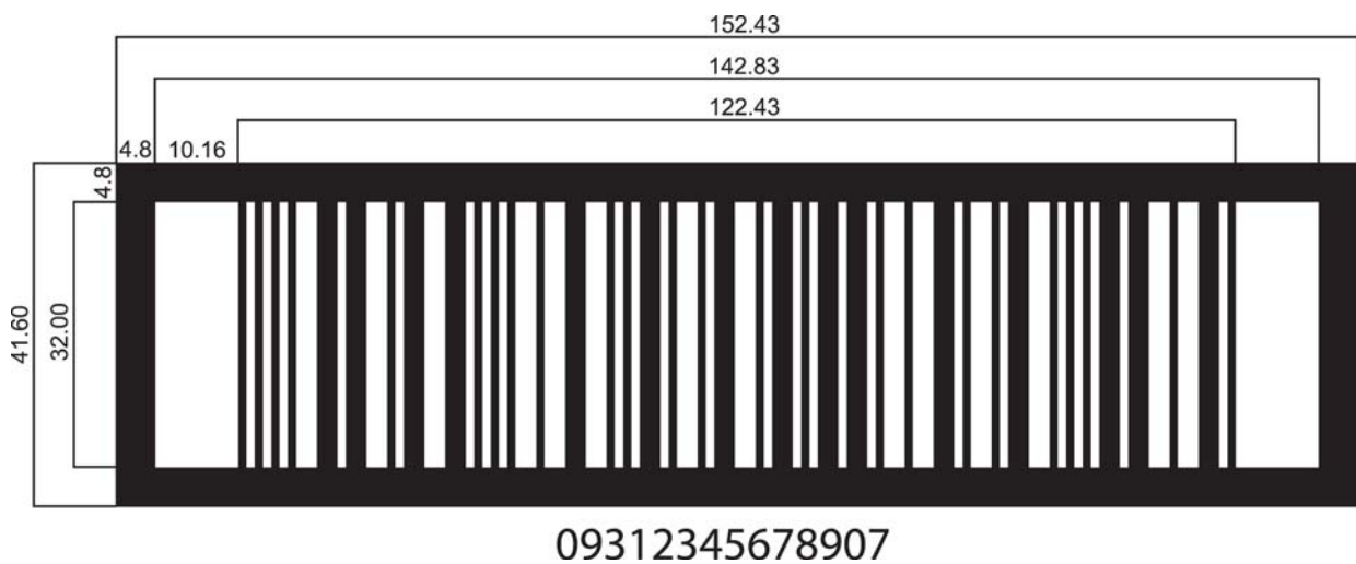
Figure 43 - ITF-14 Bar Code Nominal Dimensions
