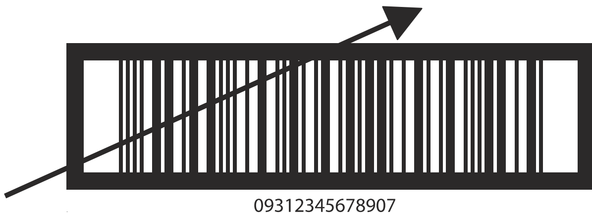
Figure 13 Example of a Skewed Scanning Beam
