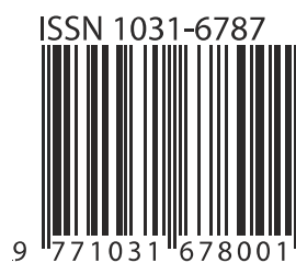
Figure 9 EAN-13 Bar Code Formed Using the ISSN
