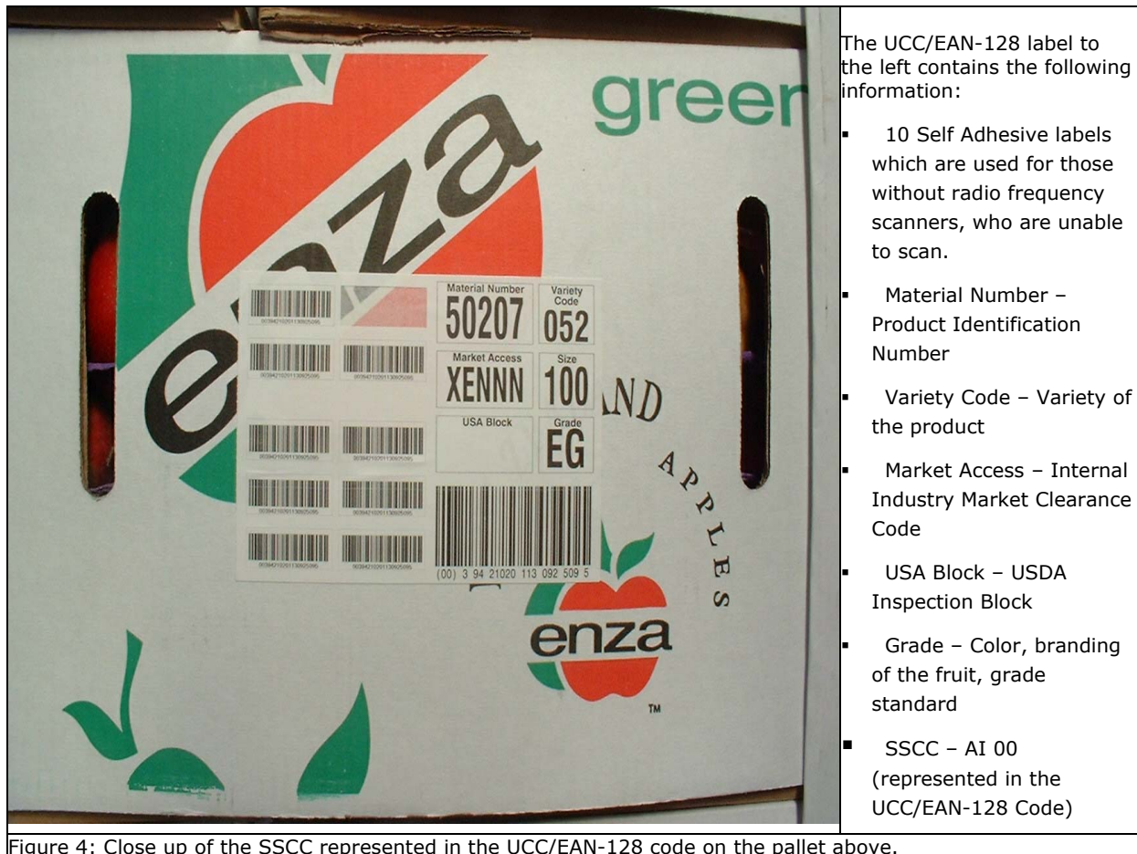
Figure 4: Close up of the SSCC represented in the UCC/EAN-128 code on the pallet above.
